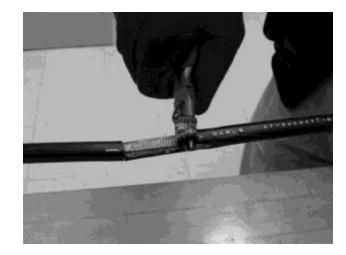
4.6 Use a pair of pliers to remove the outer sheath and expose the armor overlap (Figure 5).
