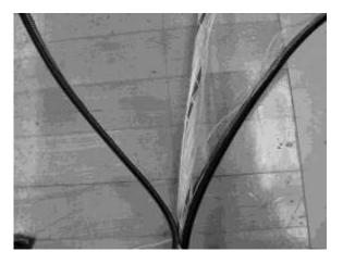
Figure 35 – Use both ripcords to remove the outer jacket.
